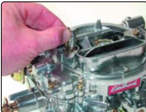
Metering rods can be changed without removing the lid from the carburetor
