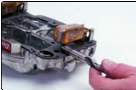
Checking float level with a 7/16" drill bit
